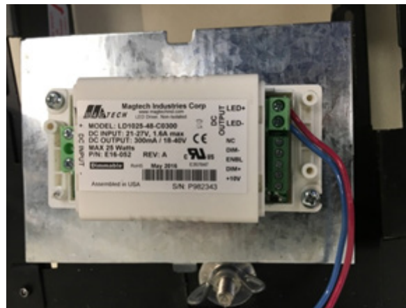
Figure D: Covers are removed from the LED driver to expose the Dimming and Power connections
